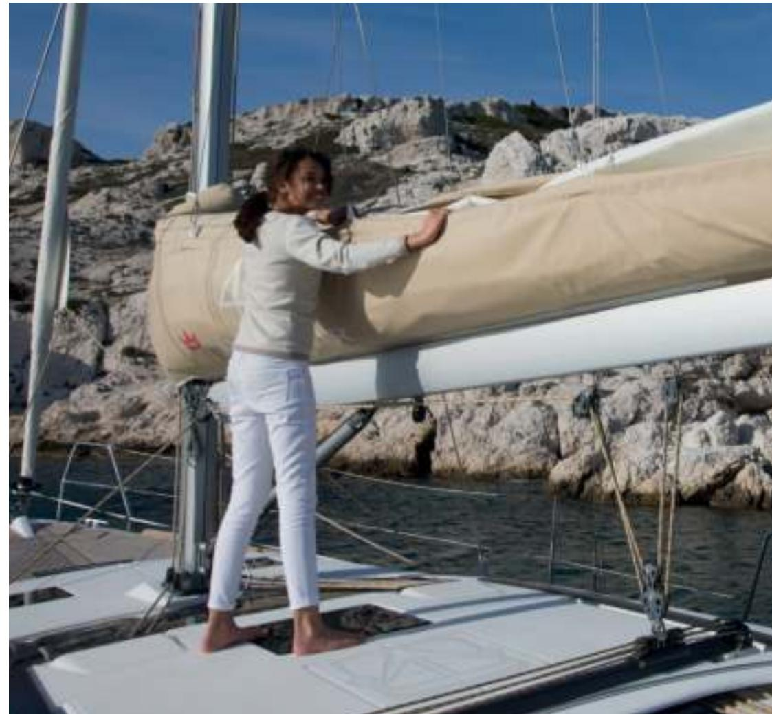
Inclined boom for easy packing
