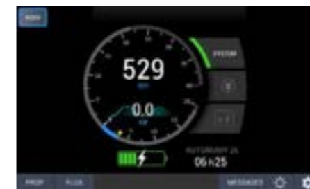
Propulsion: regeneration mode
